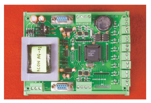
ACON AG-2 IS A DEVICE, WHICH IS USED AS A PROTOCOL CONVERTER BETWEEN TWO SERIAL DEVICES ALONG WITH EXTERNAL DIGITAL INPUTS INTERFACE FACILITY.
