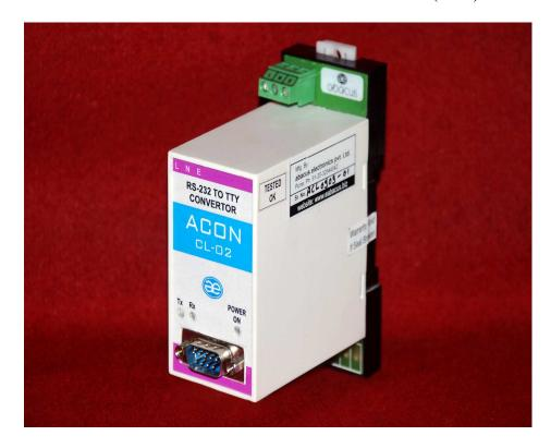
THE MODEL ACON-CL-01 IS HIGH SPEED RS 232 TO CURRENT LOOP CONVERTER. THIS CURRENT LOOP CONVERTER IS SUITABLE FOR DISTANCES UP TO 1.2 KM. OVER TWO TWISTED PAIR. THE MODEL SUPPORTS ACTIVE AS WELL AS PASSIVE PORT. (DIP SWITCH SELECTABLE).
