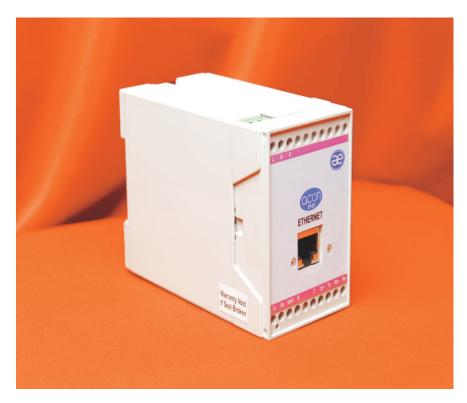
ACON ET- 01 (ETHERNET TO RS232 / RS485 CONVERTER) IS USED TO PUT DEVICES ON NETWORK SO THAT THE REMOTE DEVICES CAN BE MADE EASILY ACCESSIBLE THROUGH NETWORK COMMUNICATION.
