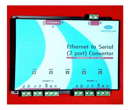
ACON ET- 02 (ETHERNET TO RS232 / RS485 CONVERTER) IS USED TO PUT DEVICES ON NETWORK SO THAT THE REMOTE DEVICES CAN BE MADE EASILY ACCESSIBLE THROUGH NETWORK COMMUNICATION.IT HAS 2 PORTS. PORT1 & PORT2.
