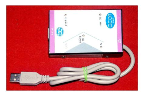
THE MODEL ACON U-02 IS USB BUS POWER, HIGH SPEED, AND USB TO RS232- CONVERTER. IT SUPPORTS AUTO BAUD RATE.
