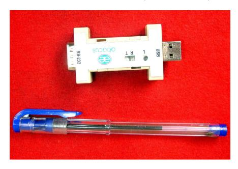
THE MODEL ACON U-03 IS USB BUS POWER, HIGH SPEED USB TO RS232- CONVERTER. IT SUPPORTS AUTO BAUD RATE.
