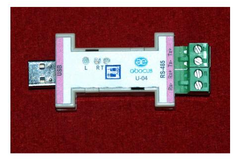
THE MODEL ACON U-04 IS USB BUS POWER, HIGH SPEED, USB TO RS485- (2 WIRE /4 WIRE) CONVERTER. IT SUPPORTS AUTO BAUD RATE.
