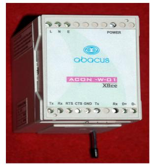
WIRELESS (XBEE) IS A SERIAL TO WIRELESS CONVERTER} THE XBEE MODULES OPERATE WITHIN THE ZIGBEE PROTOCOL AND SUPPORT THE UNIQUE NEEDS OF LOW-COST, LOW-POWER WIRELESS SENSOR NETWORKS. THE XBEE MODULE INTERFACE TO A HOST DEVICE THROUGH A LOGIC LEVEL ASYNCHRONOUS SERIAL PORT. THROUGH ITS SERIAL PORT, THE MODULE CAN COMMUNICATE WITH ANY LOGIC AND VOLTAGE COMPATIBLE UART OR THROUGH A LEVEL TRANSLATOR TO ANY SERIAL DEVICE. THE MODULE OPERATES WITHIN THE ISM 2.4 GHZ FREQUENCY BAND.
